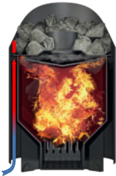
Fig. 4 Heater design and operation
